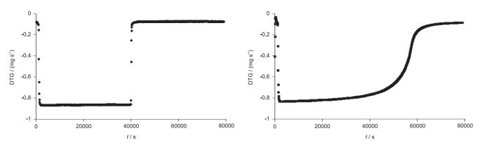
FIGURE 3. Knudsen isothermal desorption traces reported as DTG (time derivative of TG): (left) from pure water (a similar trend is observed for a saturated salt solution), (right) from a non saturated sample that modifies its composition.
