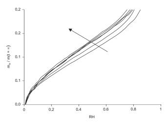
FIGURE 4. Desorption isotherms determined with Knudsen thermogravimetry for bread crumb samples of different age (from [Fessas & Schiraldi, 2005]).
